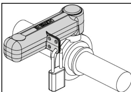
**5.** Press the two halves together until the pull handle is completely secured.
