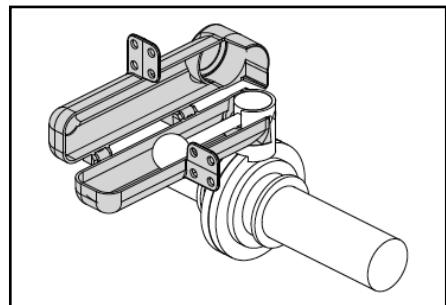
**3.** Press device against the valve shaft.
