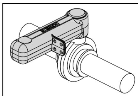
**4.** Close left side of device over the pull handle so both halves of lockout device are aligned.
